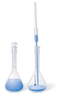
(b) The measured volume of stock solution is transferred to a second volumetric flask.
