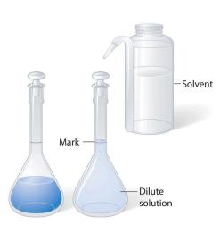
(c) The measured volume in the second flask is then diluted with solvent up to the volumetric mark  $[(V_s)(M_s) = (V_d)(M_d)]$ .
